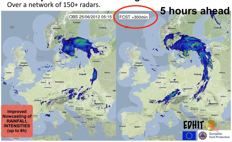
CRAHI Algorithm of nowcasting by lagrangian persistence Berenguer et al. J. Hydrometeorology, 2005; J. of Hydrology, 2011
