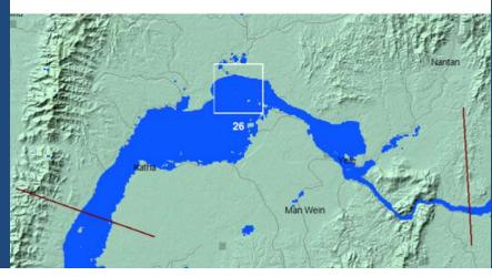
Inundation for (top) a normal winter flow, at ~200 m3/s in February 2000; (middle) normal monsoon season flow, recurrence interval of 1.1 y, ~9000 m3/s, in 2002, and (bottom) during a rare flood, recurrence interval of 21 y, 18,200 m3/s, in 2013.
