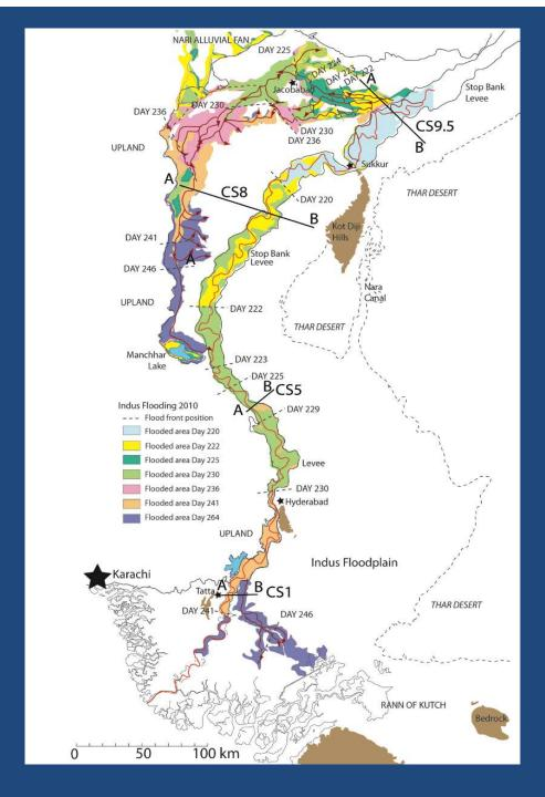
Summary map showing the progress of the 2010 Indus flood wave and its two main avulsions. Arrows and colors show the direction and dates of overbank floodwater as determined by progressive inundation from remote sensing.
