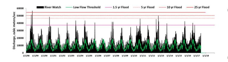
2013 39659 m3/sec 2014 29240 m3/sec 2015 42628 m3/sec Flood Frequency Analysis, 1998-2015 25 yr\* 54641 m3/sec 10 yr\* 50340 m3/sec 5 yr (major flood)\* 46626 m3/sec 1.5 yr (bankfull flood)\* 37427 m3/sec Mean Discharge 12764 \*From Log Pearson III Low Flow Threshold: 8838 m3/sec
