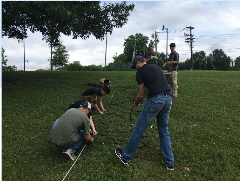
Setting up ERT cables
